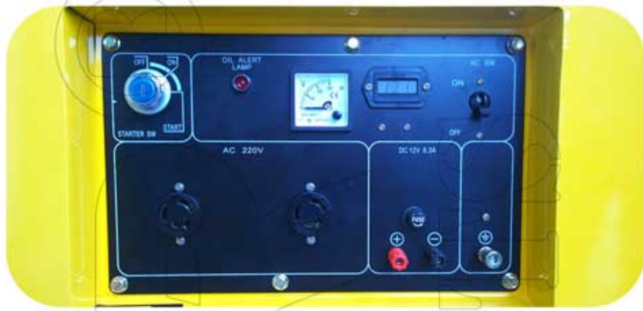
Control Panel with Hour Meter & Genset's MCCB
